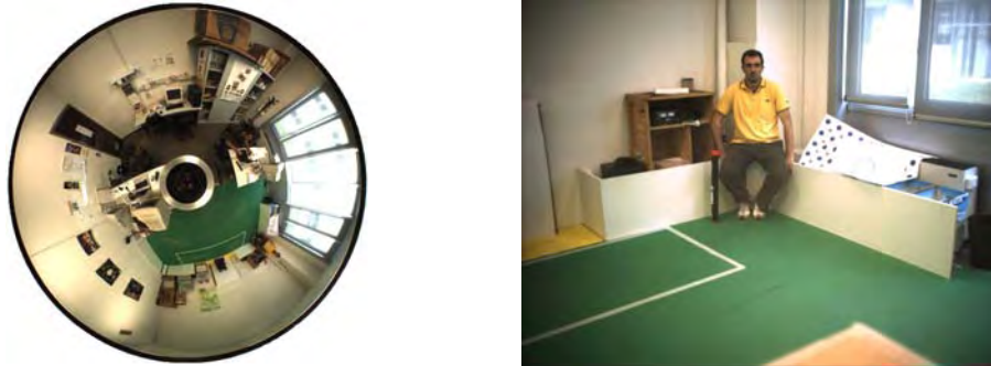
Figure 2. A pair of images acquired with the hybrid system described in (Cagnoni 2007). The omnidirectional image (left) and the perspective image (right). The different resolution of the two images is clearly visible.
