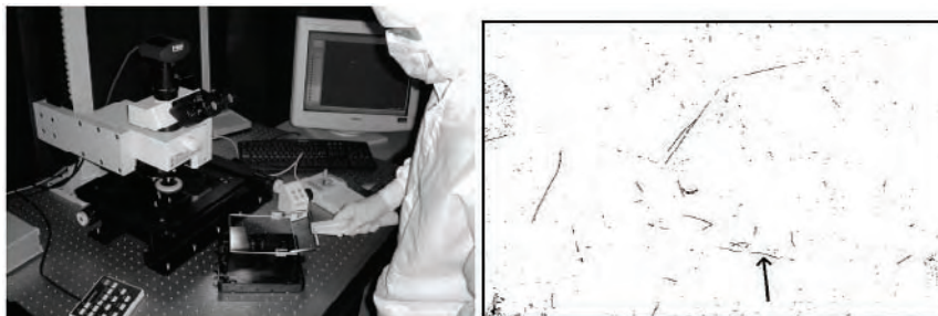
Figure 3. Automatic control system and cartography of a 100mm x 65mm optical device
